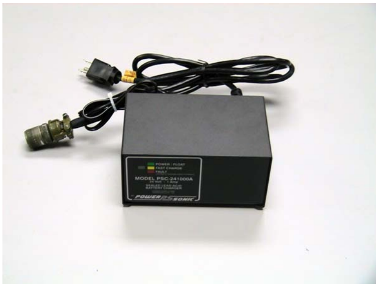
Figure 3: BC1-24V PATTERY PACK CHARGER
