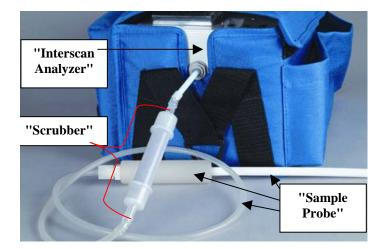
1. Creating the Sample probe assembly (P/N 030-00047) is performed by installing the scrubber (P/N 030-00046) between the sampling probe (P/N 050-00003) and the inlet of the instrument (GF1900).
